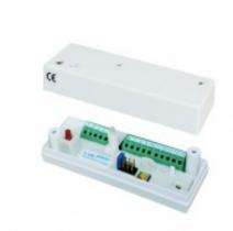
IU 400 is an interface/analyzer for glass break detector GD 475 and shock detector CD 475. It has three relays one for Intrusion, one for Fault and one for Tamper. Max 10 units of GD 475/CD 475 detectors can be connected to one IU 400 unit. **IU 400 together with GD 475/CD 475 is certified according to EN 50131-1 and EN 50131-2-7-2:2013 Grade 3, Class II**.
