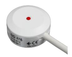
The passive glass break detector, GD475, is certified to EN Grade 3 and is suitable for float, tempered, laminated & reinforced glass. The GD475 is glued to the glass surface and will detect var-ious attacks (including cutting tools) on the glass surface. The detector requires an interface unit IU400, which senses the changes in the current characteristics of the detectors and provides alarm and fault outputs.
