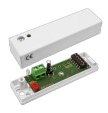
CD 475 offers reliable monitoring against attacks with mechanical tools. The CD 475 is a chock- and vibration detector with 3 separate detection channels: an integration channel / saw channel for weak signals with long duration, a counting channel that senses strong impact on the monitored surface and an explosion channel which senses very strong signals from e.g. an explosion.
